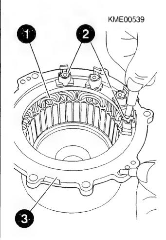
CHECKING AND REPAIRING ALTERNATOR Checking stator winding (resistance) Use alternator tester to measure stator resistance between the two outer phase contacts (1) and (2). Pay attention to measuring range on measuring instrument. Resistance value: 0,10...0,12 Ohm 0 684 201 200
